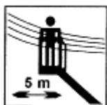
**MAI OPERARE IN PROSSIMITÀ DI LINEE ELETTRICHE AEREE AD ALTA TENSIONE E COMUNQUE IL CESTELLO DOVRÀ SEMPRE MANTENERSI AD UNA DISTANZA MINIMA DI SICUREZZA DI 5 METRI DAI CAVI** Copyright©Gruistimanovratori
